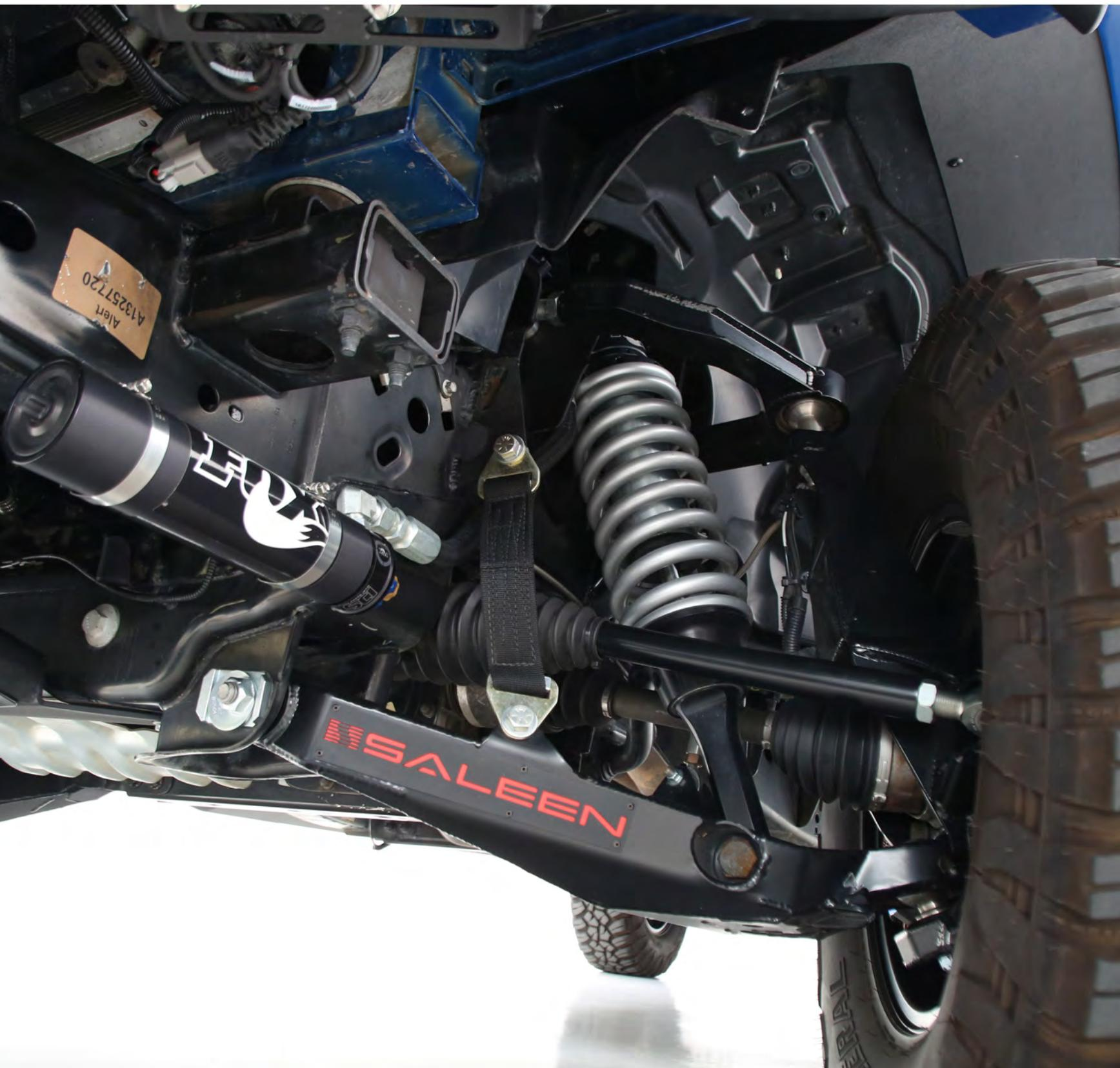
**THE FRONT SUSPENSION SYSTEM FEATURES SALEEN'S CONTROL ARMS MATCHED WITH A NEW STEERING KNUCKLE AND CUSTOM TUNED FOX 2.5 COILOVER SHOCKS**
