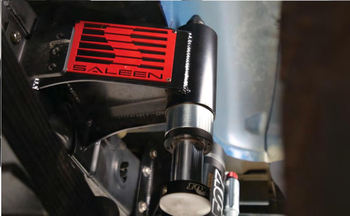
At the rear Saleen uses its own design of leaf springs, and added Fox bump stop with frame gussets to create 14-inches of travel. This is all connected to a full-floating rear axle and heavy-duty housing that is only available in the Saleen "Black Label" version of the truck, which adds the highest performance level and output available on the truck. White and Yellow Label models are also available with fewer options.
